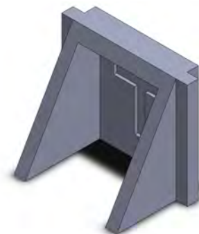
Figure 6.6: CCU Enclosure Tally CAD View
